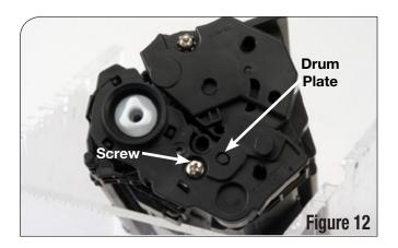
13. Using a hook tool, move the shutter torsion spring into the indent on the drum plate as shown in Figure 13. Then remove the drum plate ensuring that the drum shutter torsion spring does not get lost.
