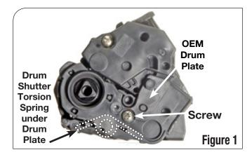
2. Using a hook tool, move the shutter torsion spring into the indent on the drum plate as shown in Figures 1 & 2. Remove the drum plate ensuring that the drum shutter torsion spring does not get lost.
